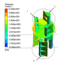
Fig. 6. Pressure distribution of wind speed is 8.5 m/s
